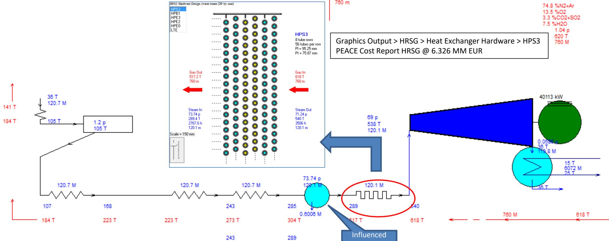
Design : 1P non reheat condensing ST, no GT, gas flow into HRSG @ 760 t/hr & 620 degC, ST inlet conditions = 69 bar & 538 deg C (@ stop valve)
